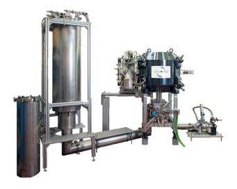
For autonomous, cheap and compact radioisotope production facility, a closed cycle cryogenic system was selected, in order to eliminate the need of periodic refills or the construction of a large cryogenic system.
